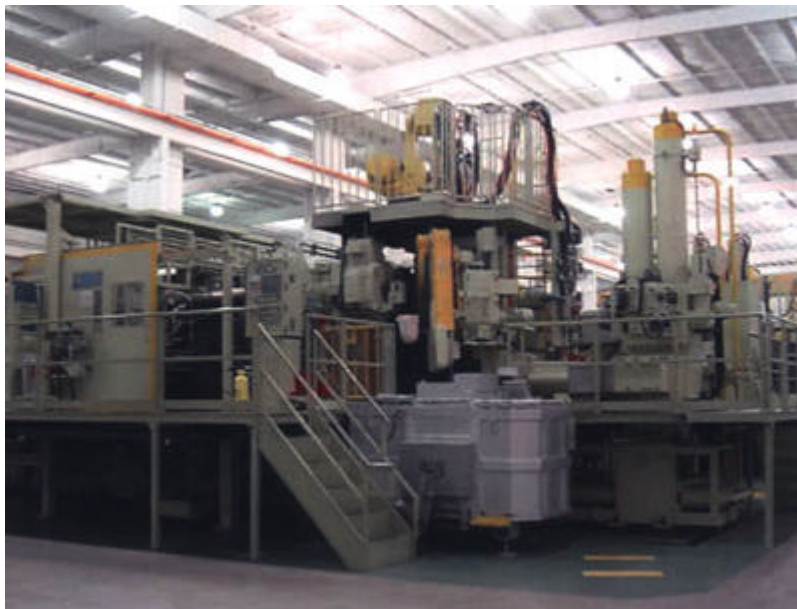
Large aluminum die-cast machine at AAC
