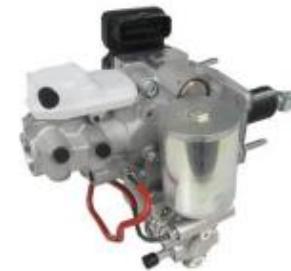
Electric-Controlled Brake System
