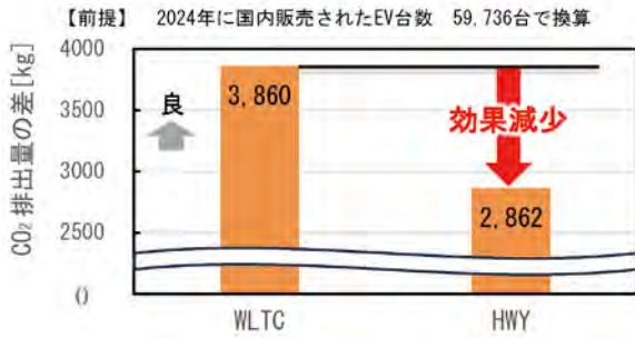
図12 Si-IGBT vs SiC-MOSFET CO 2 排出量の[kg]
