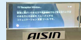
YY Reception Window, a transparent display enabling conversation while looking at the face of the other speaker
