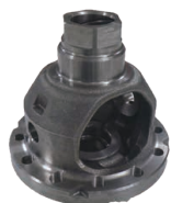
Thin differential casing achieved through the development of high-strength materials
