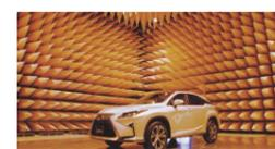
Evaluation of electromagnetic waves transmitted to electronic devices
