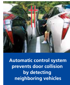
Automatic control system prevents door from opening
