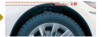
The vehicle rises to a height that facilitates easy entry (+30mm).
