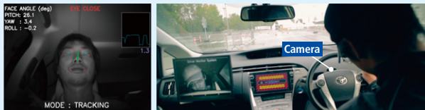
This technology detects any abnormalities with the driver based on facial direction and the degree to which the driver’s eyes are open and safely guides the vehicle to the road shoulder.
