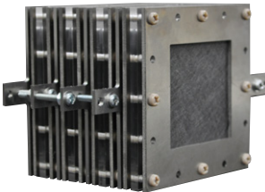
Prototype of the rechargeable lithium-ion battery stack (four-cell)
