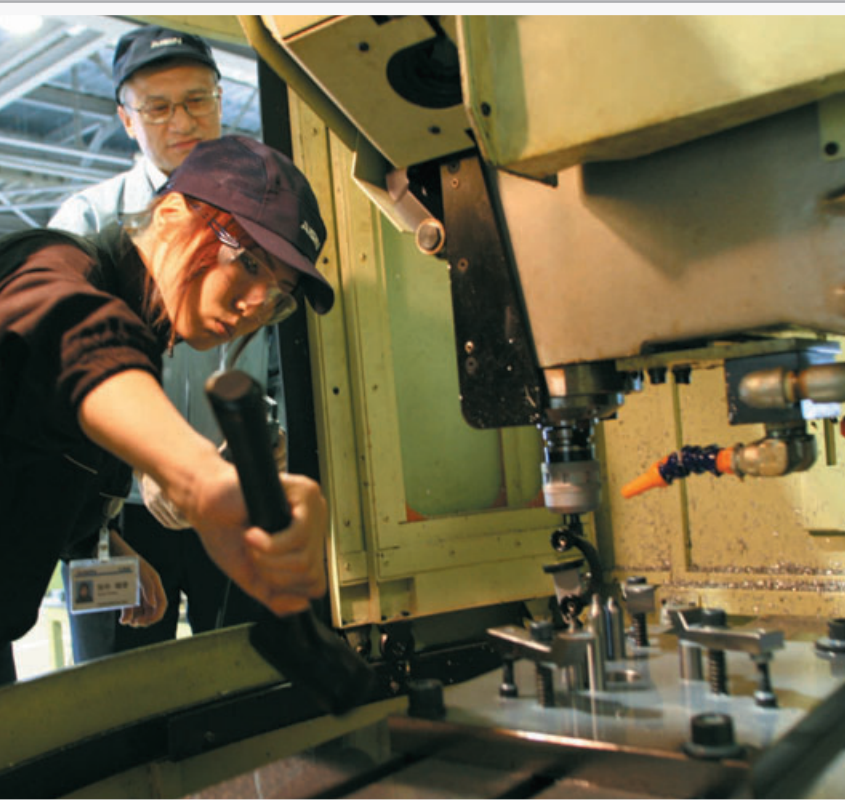
Experiencing jig and blade replacement, program creation and cutting at the machining center in the Back-to-Basics “Mono-zukuri (manufacturing)” Workshop.
