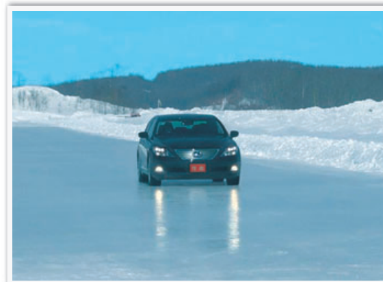
Reliability testing through brake performance evaluation on a freezing surface
