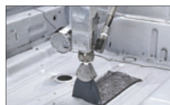
Spray-type damping coat
