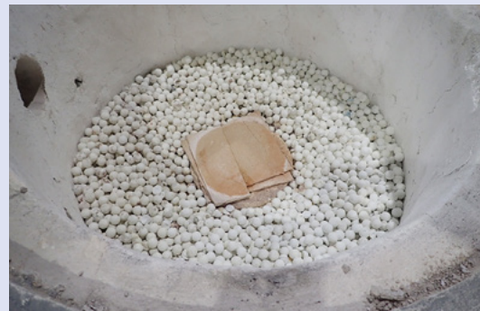
Hearth of the holding furnace
