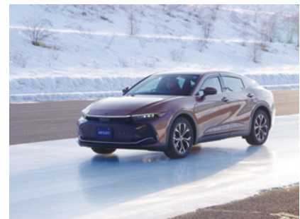
Handling stability road-testing on artificial ice
