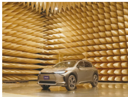
Assessment of electromagnetic interference on electronic devices
