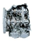
Small Torque Capacity CVT
