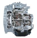
High Torque Capacity FWD 8-Speed Automatic Transmission
