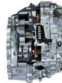
High Torque Capacity FWD 2-motor hybrid transmission
