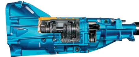
Medium Torque Capacity RWD 6-Speed Manual Transmission
