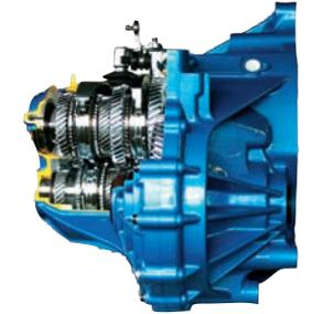
High Torque Capacity FWD 6-Speed Manual Transmission
