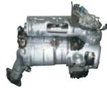
Exhaust Manifold & Converter
