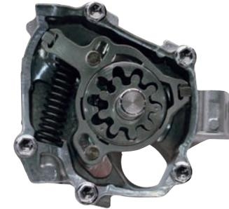
Continuously Variable Capacity Oil Pump
