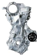
Engine Front Module (timing chain case with water and oil pumps)
