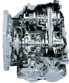
Small Torque Capacity CVT
