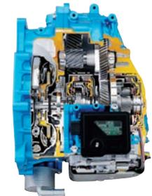
Medium Torque Capacity FWD 6-Speed Automatic Transmission
