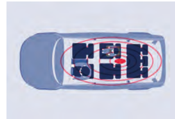
Detecting an infant left alone in the vehicle with a single sensor
