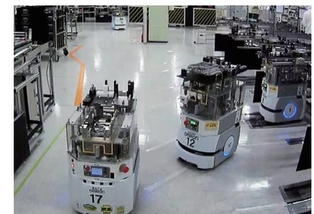
This system obtains the production status, the operation status of automated guided vehicles (AGVs), etc. in real time to generate and distribute the optimal conveyance plan based on the obtained information, thereby achieving autonomy conveyance with AGVs.
