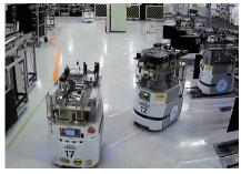
This system obtains the production status, the operation status of automated guided vehicles (AGVs), etc. in real time to generate and distribute the optimal conveyance plan based on the obtained information, thereby achieving autonomy conveyance with AGVs.
