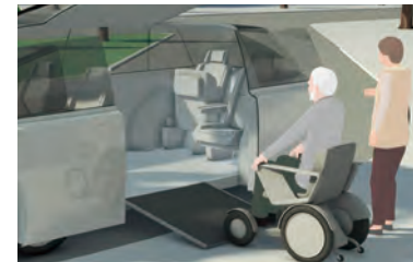
Large-opening doors combined with an electric ramp for smooth entry and exit
