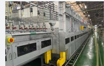
Continuous furnace for battery heat sinks
