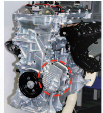
▶▶ The first automotive electric water pump for cooling the engine successfully developed in Japan
