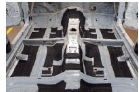
High-performance spray damping coat
