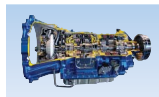
6-speed AT for light-duty compact commercial vehicles
