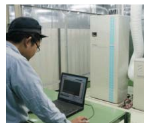
Performance testing of fuel cells for home use
