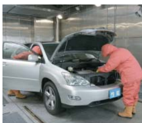
Engine start-up and other vehicle performance testing are conducted in a cold-weather chamber at temperatures as low as -50°C
