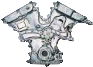
Engine front module reduces vehicle weight and costs using combined components
