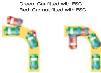
ESC ensures stability of automobile during cornering
