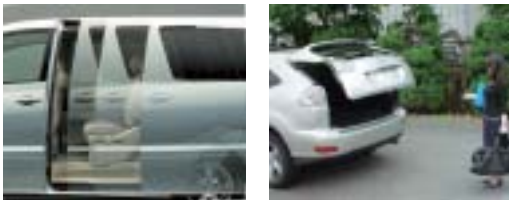
Power sliding door and power back door systems easily open and close by remote control
