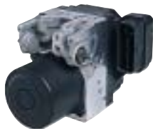
Quiet brake modulator employed in ESC
