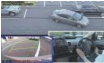
Intelligent Parking Assist fitted in the Toyota Prius
