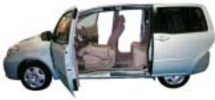
Center pillarless door latch system fitted to Toyota Raum
