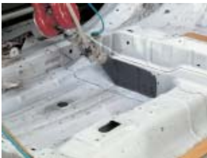
Spray type damping materials absorb car vibrations through use in floor boards
