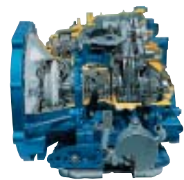
CVT using control technology expertise accumulated during AT production
