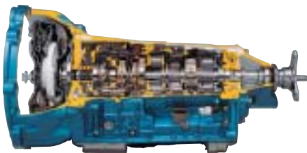
Newly developed RWD 6-speed AT fitted to the Toyota Celsior (LEXUS LS430)
