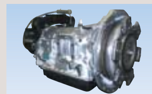
6-speed ATs for light-duty trucks and buses
