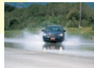
Vehicle stability control system is evaluated on a low-friction \mu surface road.
