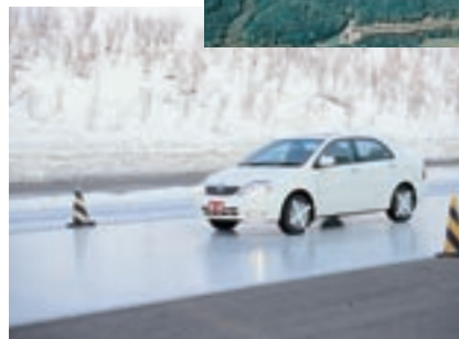
Braking test on a frozen road.
