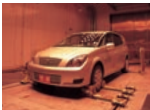
Various vehicle components are evaluated in a hot-weather chamber of temperatures up to 50°C.
