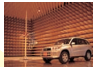
Effects of electromagnetic waves upon electronic devices are evaluated in an anechoic chamber.
