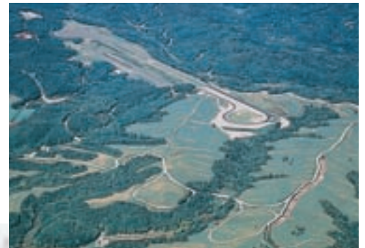
Toyokoro Proving Ground (Hokkaido) Land area: 7,480,000m 2 High-speed track: 2.2km/lap Rough road track: 11.5km/lap
