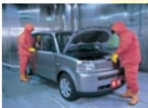
Function and performance of vehicle components are tested in a cold-weather chamber of temperatures down to -50°C.
