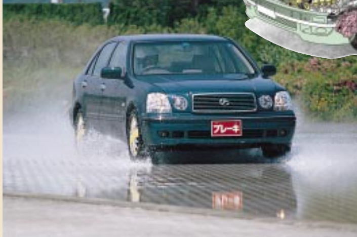
Stability Control System Performance evaluation tests
